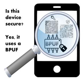
A BPUF can be added to any electronic device, either by including a firmware that exploits intrinsic hardware of the device (SRAM, for example) or by including a dedicated hardware block in the device.
