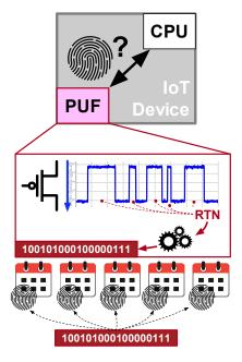
An aging-resilient identity can be obtained from the RTN present in the current of just a single transistor.
